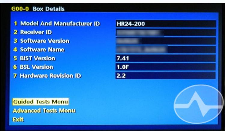
If you want to do some more advanced testing of the receiver, reboot it and press {SELECT} when you see “Running receiver self-check.” This will take you to a very advanced test menu that will let you test almost every aspect of the receiver and give you at least a pass/fail. *This test will also give you the power to erase your hard drive, so be careful.*
