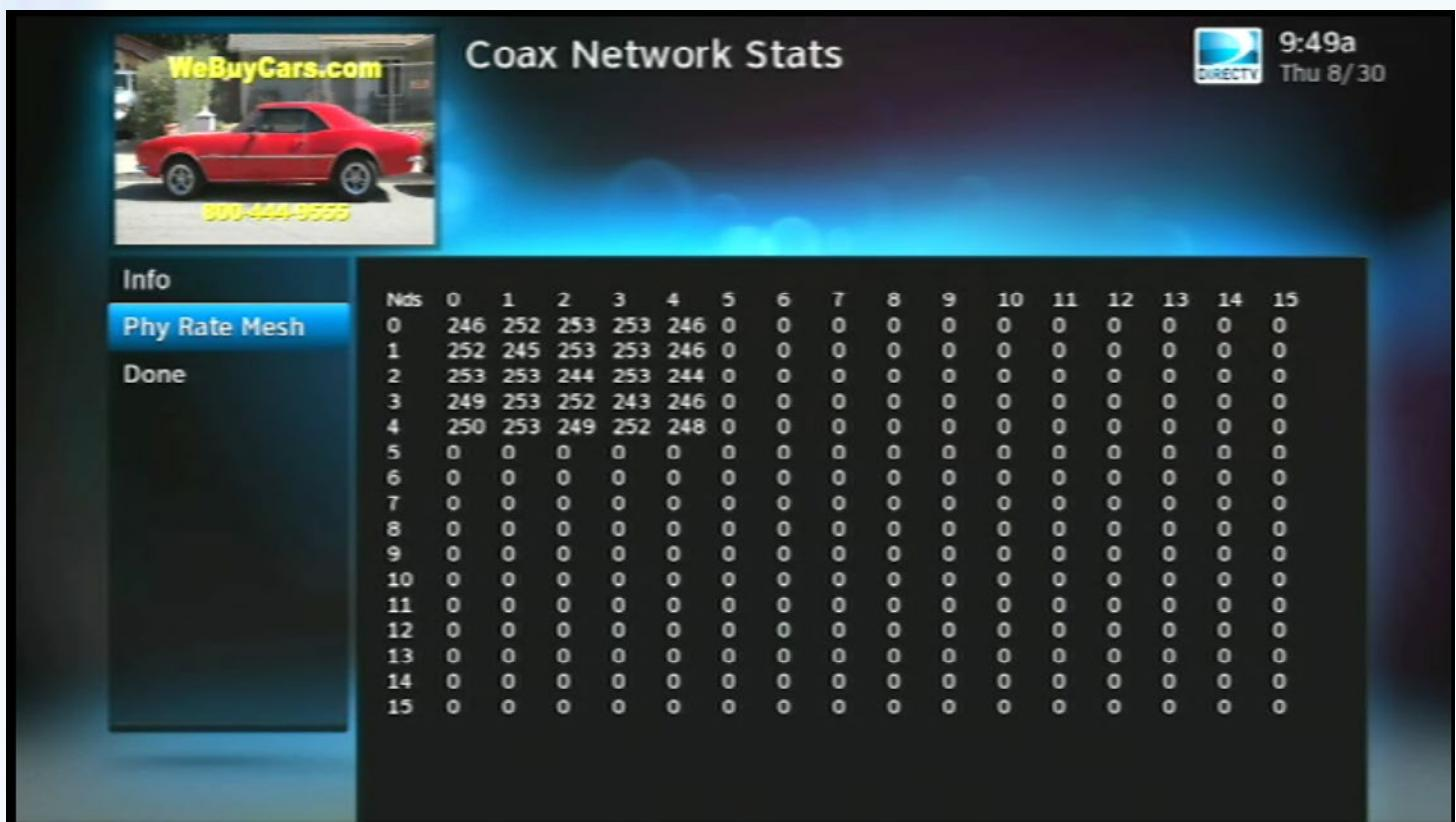
When you're ready to get really deep into figuring out the problems with your network, it's time to look at the Phy Rate Mesh test. This tests the communication between everything in your network. Before you go into that test, write down the node ID's, as you will need them to the next test. Then arrow down to "Phy Rate Mesh" and press {SELECT}.
