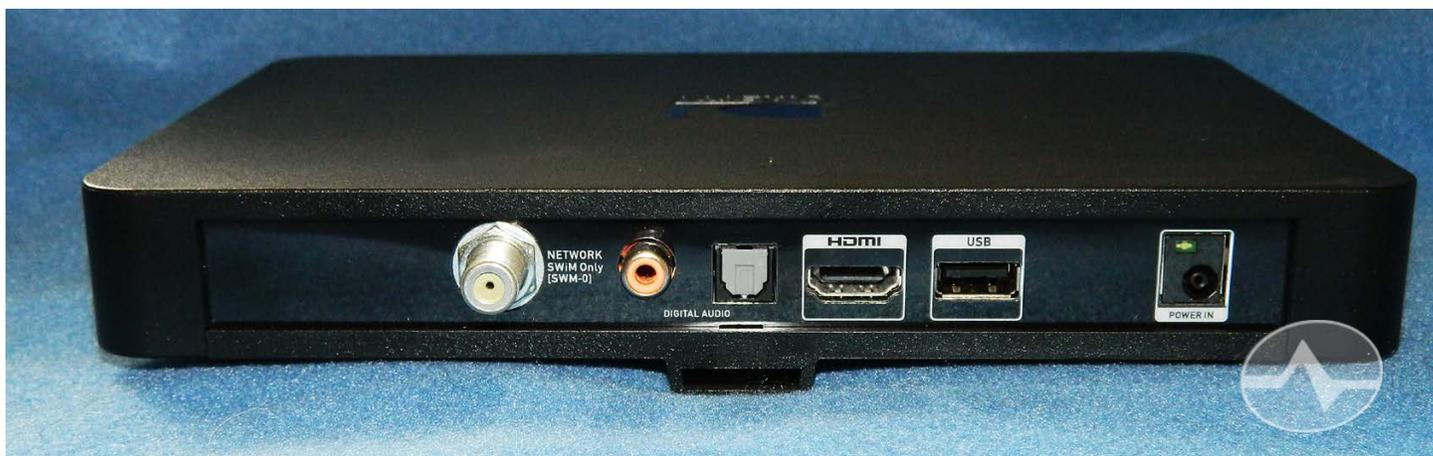
The good news is that the C61K has a full complement of outputs. The HDMI output is fully HDMI 2.0/HDCP 2.2-compliant, and there are both optical and coaxial digital outputs. DIRECTV puts a USB port on everything, and in this case it won't do much for the software. It's a convenient place to plug in the power from a streaming stick, and that's about it.
