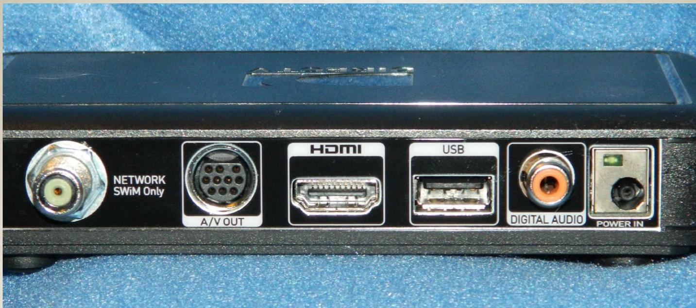
Even though this receiver is tiny, there's a lot going on behind it. Of course, there's a coax input. Because the HR34 is SWM-only, and because you need an HR34, this box is SWM-only too. The next connector is for a component or composite connection. Our [H2510PIN](#) dongle for H25s works fine, and there will be one for composite as well.
