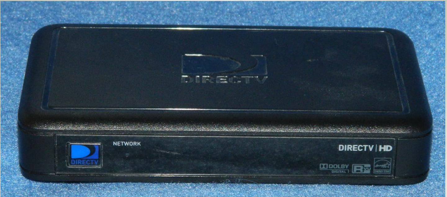
There's not a lot to look at with this little box. The front panel has one button on it. Quite a change from the old days when there were 15 or more buttons on the front. It will work with an RF or IR remote, but you do have to use a remote. The power button lights up when the C31 is in use. To the right of it is a network light that glows green when the C31 is connected to an HR34.
