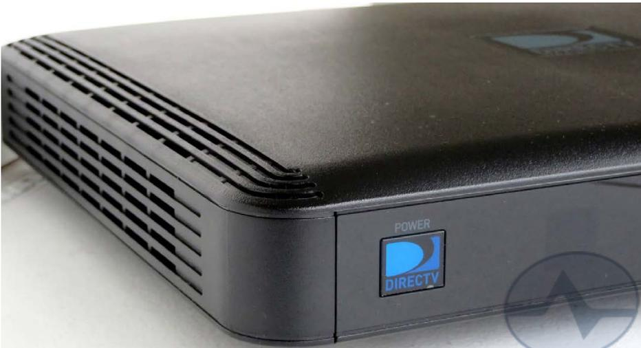
The HR54 has most of the same capabilities as the HR44, but does away with several obsolete and unnecessary parts in the interest of speed. Externally it's a very close cousin to the HR44, but don't try to use the front buttons. Gone is the touch-sensitive front panel, replaced by a single physical button similar to that found on the C41 Genie Mini Client. There's a record light just to the right, but the rest of the front panel is nothing but sheer black.
