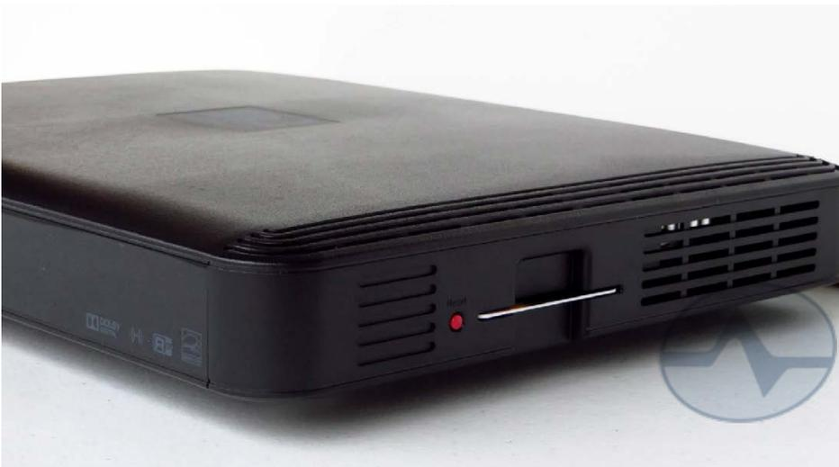
The access card and reset button have been relocated to the side, and the front loses its (useless) USB port.
