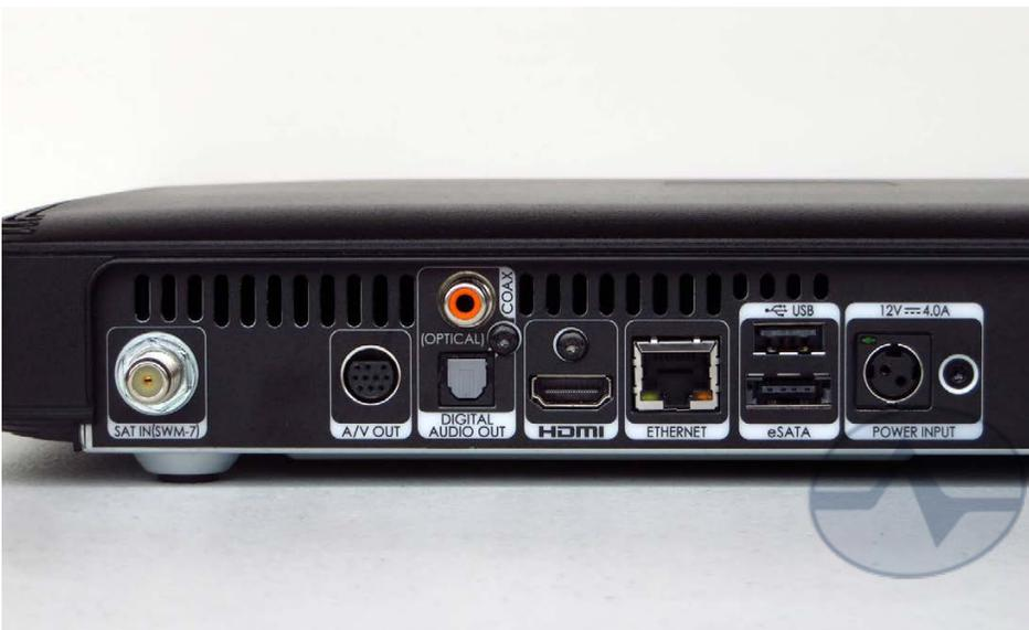
The component and composite connections from the HR44 are gone, replaced by a single connector. This 10-pin jack can be used for the **H2510PIN** or **10PINCOMPOS** cables if you do need to connect another TV. Luckily, optical audio still remains, as does the USB connector for the AM21 antenna module. The HR54 uses the same EPS44 power supply as other Genie DVRs.
